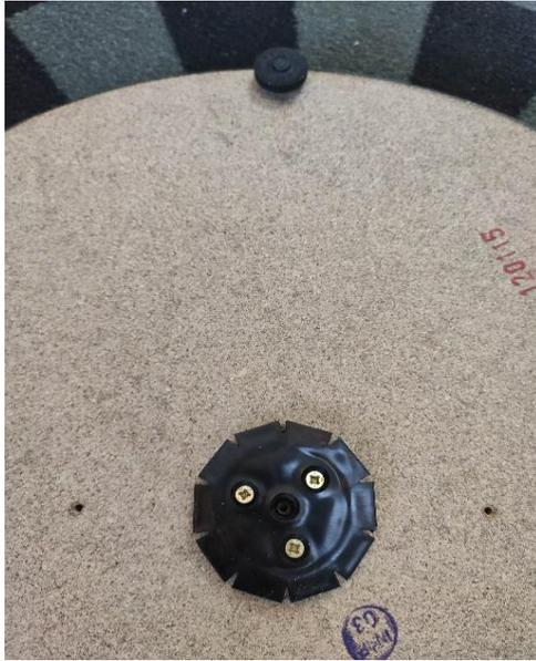
*Figure 2: Attach the board mount*
