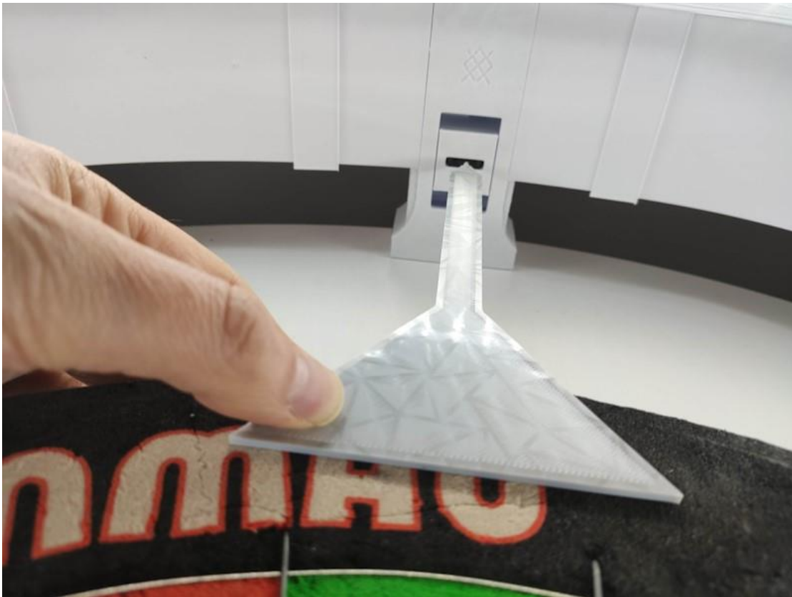
Figure 4: The tip of the camera height tool should be at the same height as the black aperture of the camera holder
