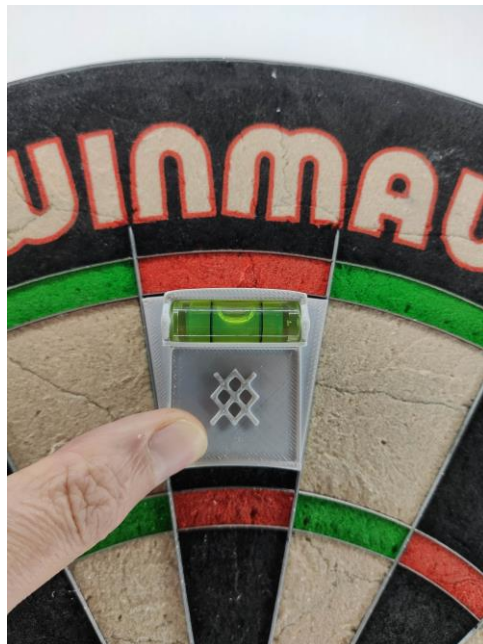
Figure 3: The board must be level after the board mount is attached
